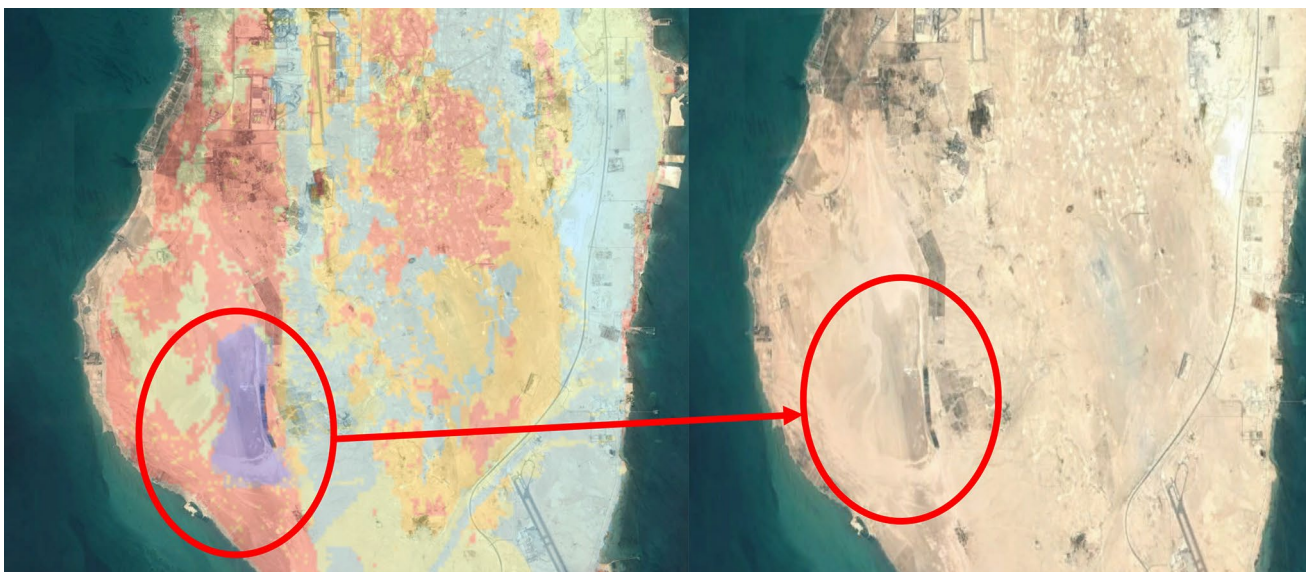
Fig. 10 Optimal location for the aquifer recharging as resulted from the MCDM and GIS techniques in Google Earth
