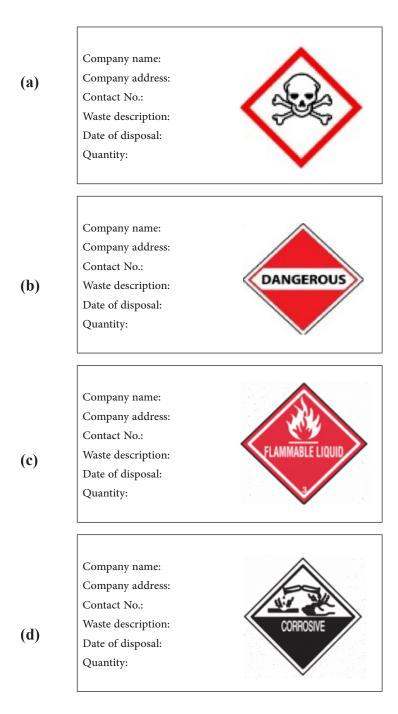
Figure 1: The format of the label sticker that should be presented on the container of (a) reactive waste, (b) solid hazardous waste, (c) used oil and (d) corrosive waste.
