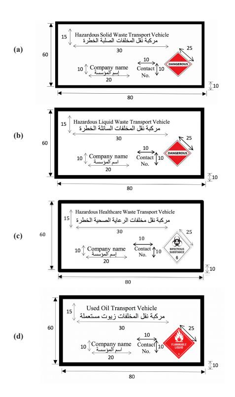
Figure 2: Detailed format of the hazardous (a) solid waste, (b) liquid waste, (c) healthcare waste and (d) used oil transport vehicle side, showing the exact location of the labelling and the placard.
